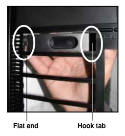
2. Press the dummy cover into the slot opening until the hook tab clicks in place.
